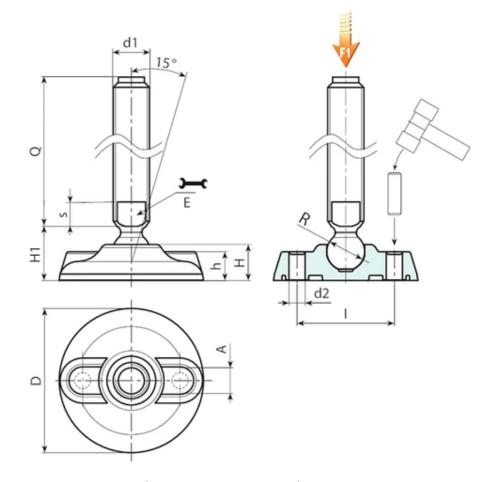
Version P912: Mounting foot with stem type B (with milled seat for wrench) and ball 12.4
