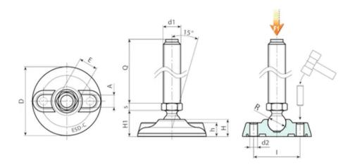
Version P911ESD: Mounting foot with stem type A (with hexagonal base) and ball 12.4
