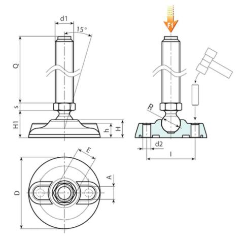
Version P911: Mounting foot with stem type A (with hexagonal base) and ball 12.4
