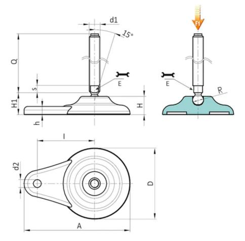
Version P704: Teardrop mounting foot with ground fixing - stem type B (with milled seat for wrench) and ball 12.5
