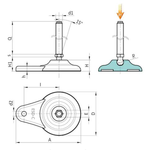
Version P700ESD: Mounting foot with stem type A (with hexagonal base) and ball 12.4
