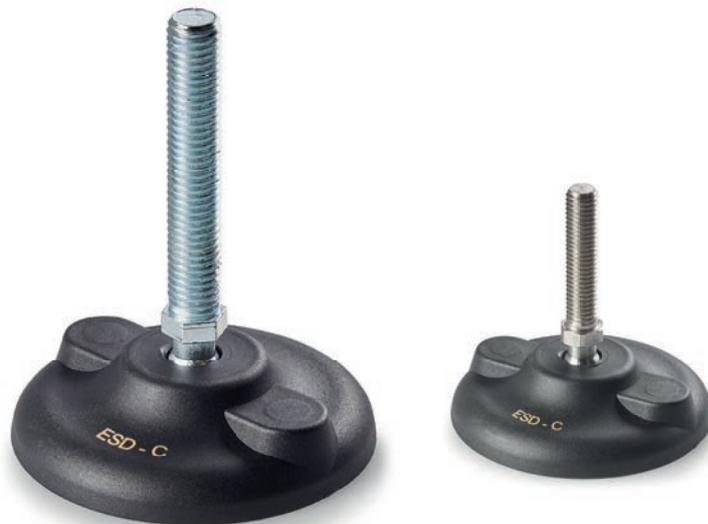
**Notes:** This item is made from ESD-C (Electro Static Discharge - Conductive) material with fillers in compliance with standards EN 100015/1 and IEC 61340-5-1. The product is conductive and prevents the formation of electrostatic discharges by facilitating its grounding. A yellow pad-printed symbol (ESD-C) enables correct identification of the product. Product suitable for the production of electronic material and for use in explosive atmospheres.
