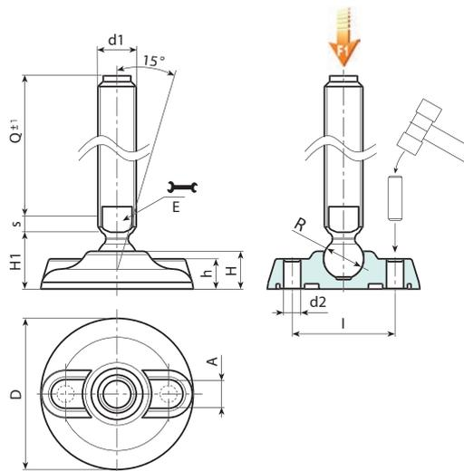
Version P912: Mounting foot with stem type B (with milled seat for wrench) and ball 12.4
