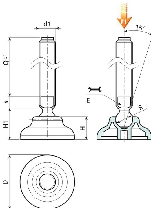
Version P906: Mounting foot with stem type B (with milled seat for wrench) and ball 12.4
