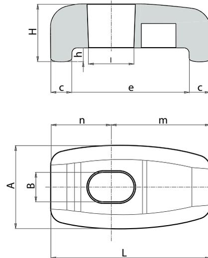
The use of the J300 bracket must be combined with a knob with a threaded stud. An effective combination could be the one with T-handle art. L271. Used together they function as a quick locking and release system for panels of machinery in general. Particularly suitable for insulating panels of large external air conditioning chiller units.
