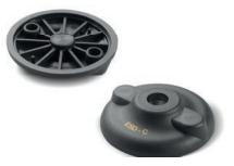
Notes: This item is made from ESD-C (Electro Static Discharge -Conductive) material with fillers in compliance with standards EN 100015/1 and IEC 61340-5-1. The product is conductive and prevents the formation of electrostatic discharges by facilitating its grounding. A yellow pad-printed symbol (ESD-C) enables correct identification of the product. Product suitable for the production of electronic material and for use in explosive atmospheres.
