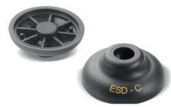
Notes: This item is made from ESD-C (Electro Static Discharge – Conductive) material with fillers in compliance with standards EN 100015/1 and IEC 61340-5-1. The product is conductive and prevents the formation of electrostatic discharges by facilitating its grounding. A yellow pad-printed symbol (ESD-C) enables correct identification of the product. Product suitable for the production of electronic material and for use in explosive atmospheres.
