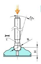
Version P542: Galvanised steel mounting foot with stem type B (with milled seat for wrench) and ball R12.5 - with SBS non-slip base
