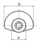
This cam can be used in combination with any handwheel with stud. In this way, as illustrated in the sketch to the side, the assembly becomes a simple latch for securing doors. Turning the handwheel also rotates the cam, which, being a spiral shape, varies the grip thickness to latch onto the door.
