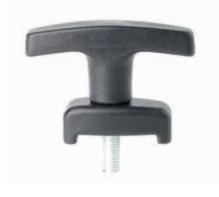
The use of the J300 bracket must be combined with a knob with a threaded stud. An effective combination could be the one with T-handle art. L271. Used together they function as a quick locking and release system for panels of machinery in general. Particularly suitable for insulating panels of large external air conditioning chiller units.
